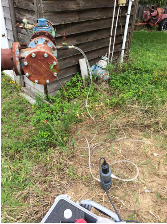
Figure 4. Examples of in-field well sampling methodology. A hose is connected to a spigot and water is routed through tubing attached to a YSI multi-probe low-flow sampling port. The YSI probe continually measures water temperature, specific conductivity, pH, and total dissolved solids. When these parameters stabilize, samples are collected in prepared containers from tubing exiting sample chamber.
