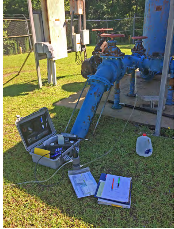
Figure 4. Examples of in-field well sampling methodology. A hose is connected to a spigot and water is routed through tubing attached to a YSI multi-probe low-flow sampling port. The YSI probe continually measures water temperature, specific conductivity, pH, and total dissolved solids. When these parameters stabilize, samples are collected in prepared containers from tubing exiting sample chamber.
