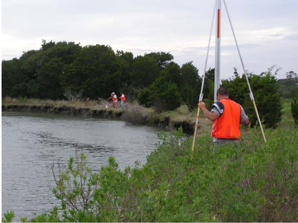
Figure 12. South Carolina Geodetic Survey leveling of stage stations.
