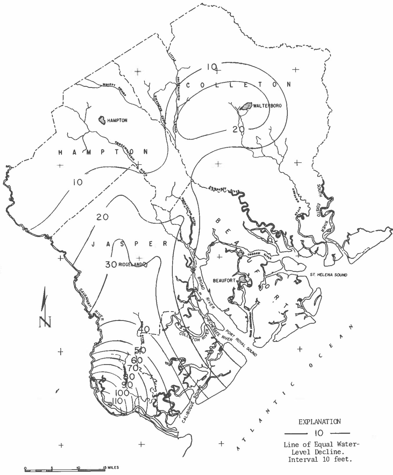
FIGURE 13. MAP SHOWING TOTAL WATER-LEVEL DECLINE IN THE TERTIARY LIMESTONE AQUIFER, 1880-1976 (AFTER HAYES, 1979).
