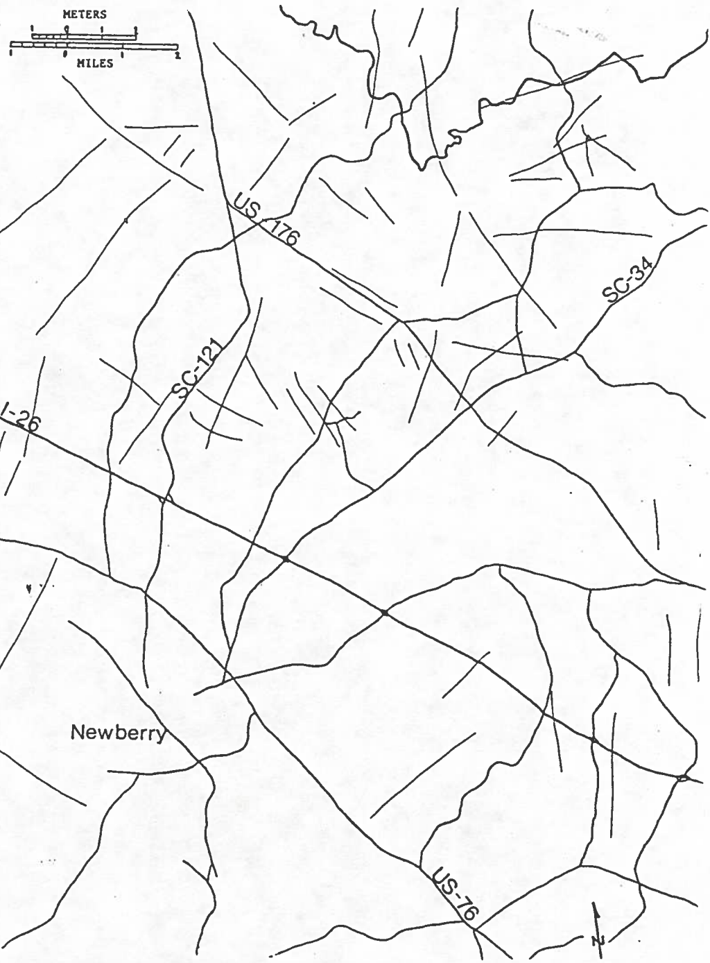
Figure 5. Multi-spectral SPOT "pseudo-stereo" lineaments over Hellers Creek area.
