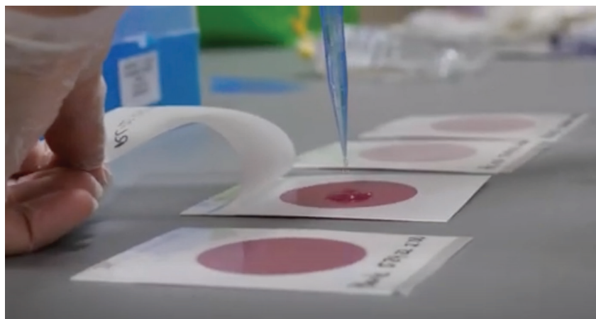
Lift the top film of the plate by a corner and release 1 ml of your sample onto the pink circle. Be careful not to touch the circle with the pipette tip or your hand.
