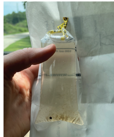
Discard and resample if sediment is stirred up and collected in the sample bag.
