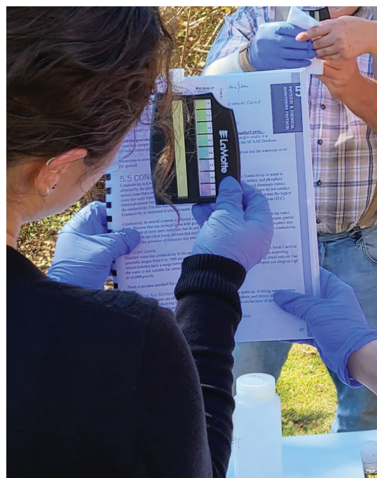
It's often helpful to use a white background when comparing your pH sample to the Octa-Slide bar.
