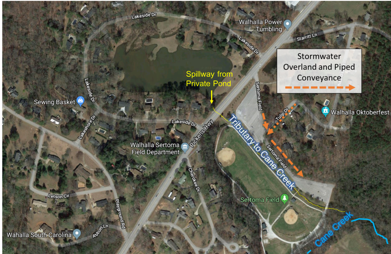
Fig. 21. Sertoma Field and conveyances of runoff and pond input to Cane Creek.
