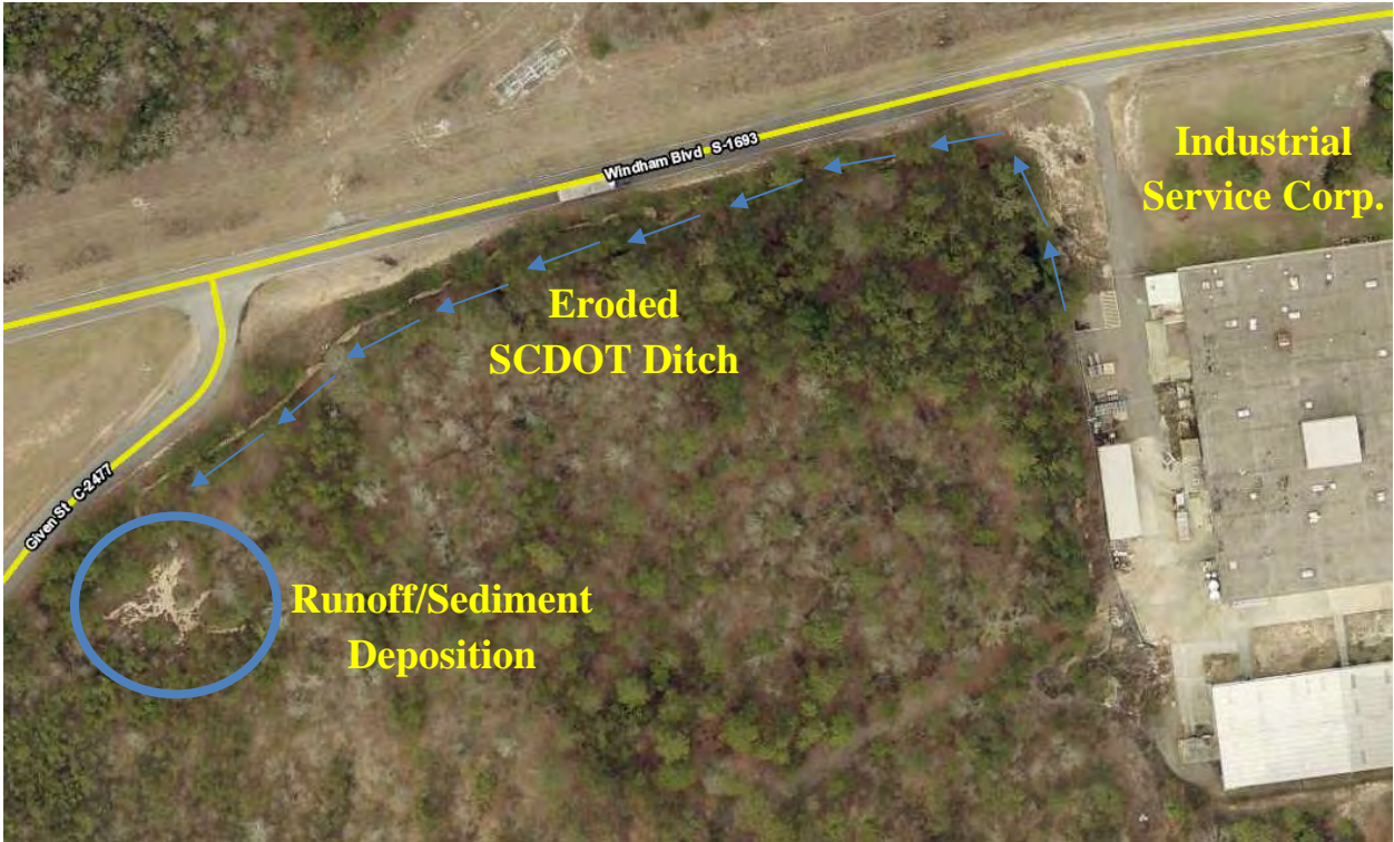
Figure 10. Eroded SCDOT Ditch down gradient from Industrial Service Corp. along Windham Blvd.
