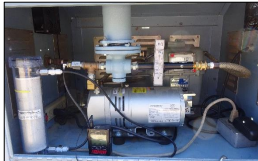
Example of an Air Monitoring Station with Rain Collection Pan and Glass Fiber Filter (on top) and Silica Gel Column (inside)
