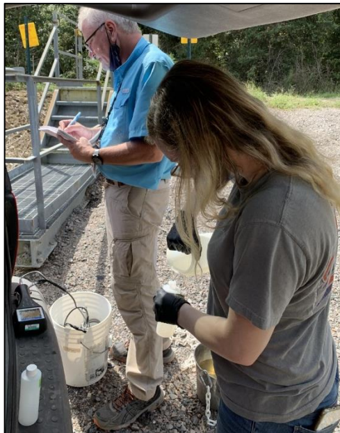
Recording field parameters: DO, pH, temperature, conductivity, and total dissolved solids
