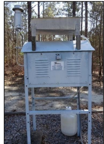
Example of an Air Monitoring Station with Rain Collection Pan and Glass Fiber Filter (on top) and Silica Gel Column (inside)
