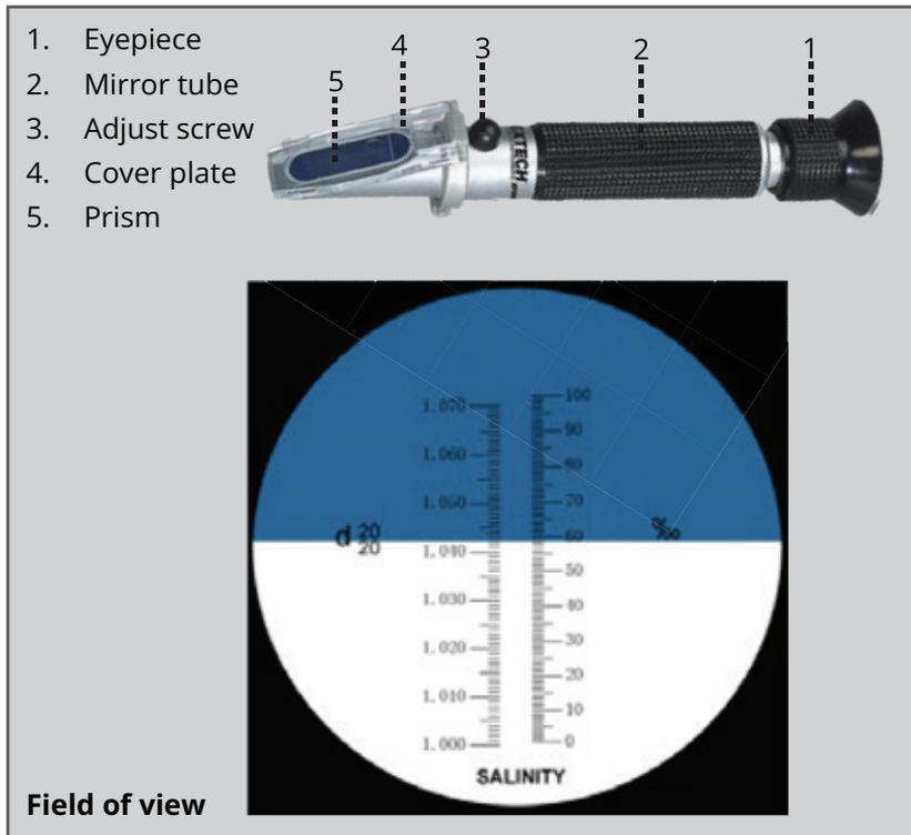
Parts of a refractometer.
