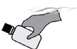
Tightly cap the bottle, and submerge it to the desired depth.
