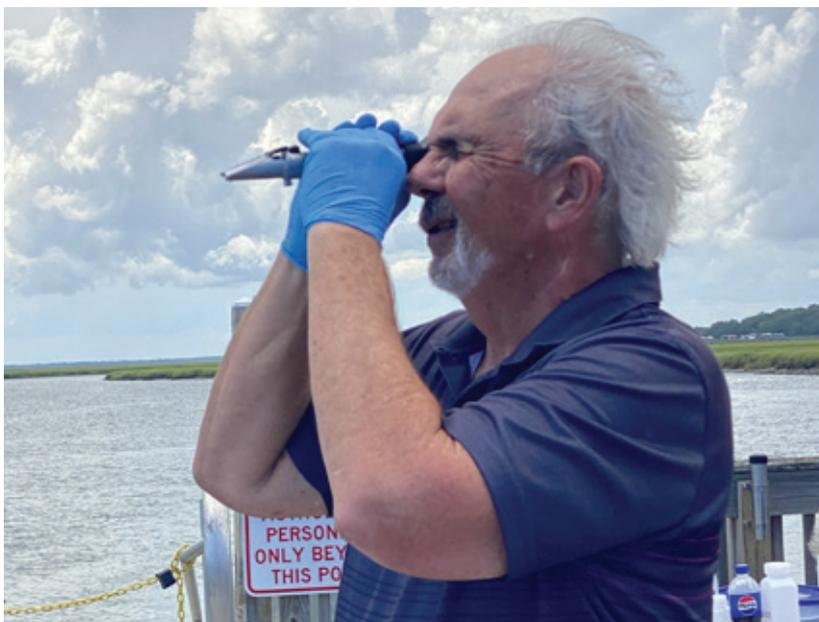
Using a refractometer to measure salinity.
