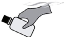
Replace the cap while the bottle is still submerged.
