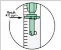
Read the syringe from the bottom of the green ring. In this example, the result is 4.0 mg/L or ppm.
