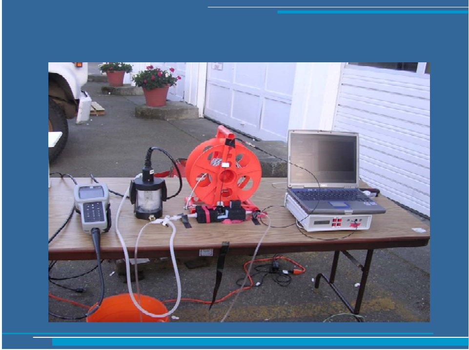
Figure 4-3. Flow-through cell set up at 8MW47
