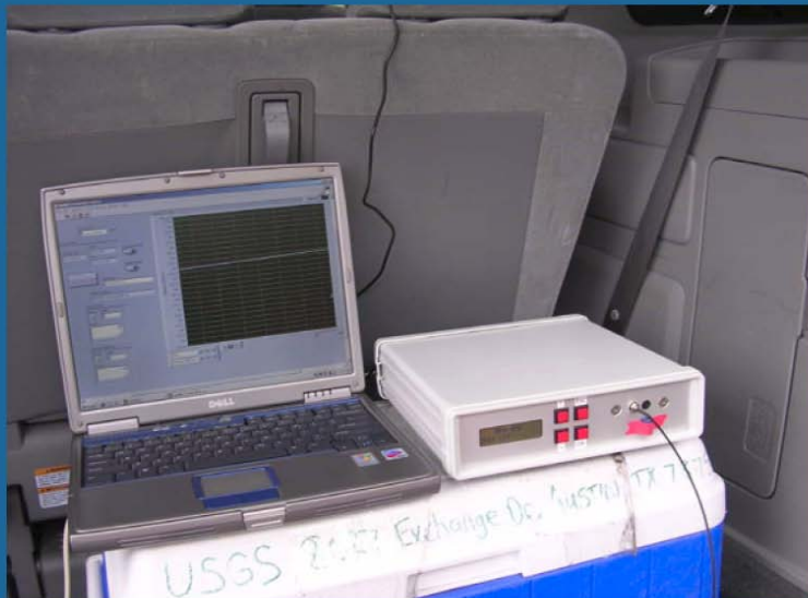
Figure 14. Flow-Through Cell Readout Setup.
