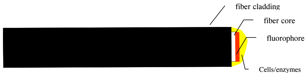
Figure 6. Fiber-Optic Biosensor. (One end of the optical fiber is coated by a pH-sensitive fluorophore, which in turn is covered by cells or enzymes entrapped in Ca-alginate.)
