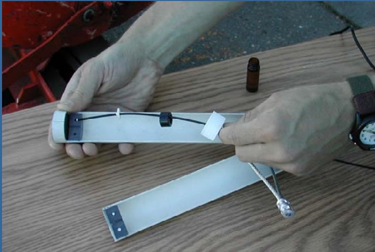
Figure 4-12. Down-hole profiling setup.
