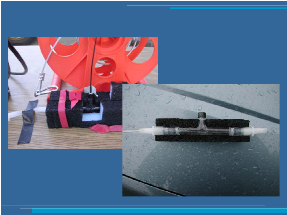
Figure 4-2. Flow-through cell set up
