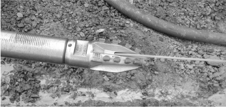
“All Soils” Spade Bit and Mud Jet
