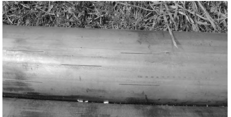
Longitudinally Slotted 304 SS Pipe
