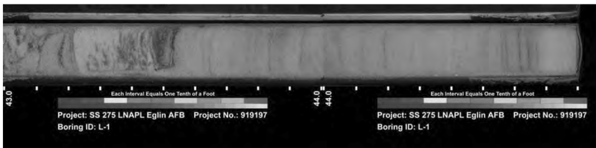
Figure 2 Digital Photograph of Intact Soil Core Segment
