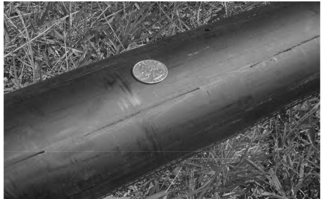
Typical Air Sparge “Screen” (Slotted Pipe): 4” HDPE Pipe, 400 ft Long Slotted Section 0.020 Inch Wide Slots, <0.5% Open Area
