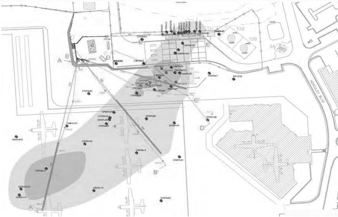
Petroleum Plume. Four Blind End HDPE Sparge Wells, Each ~ 350-600'
