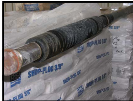
Lower inflatable bladder of packer assy.
