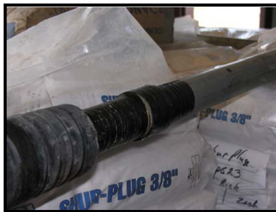
Inflatable bladder (left) water intakes (right)
