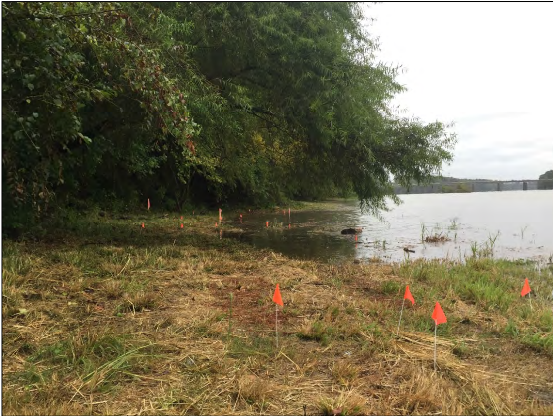
9/24/2015 – View from the Alluvial Fan looking towards the southern FDP area. Orange flags represent located magnetic anomalies.
