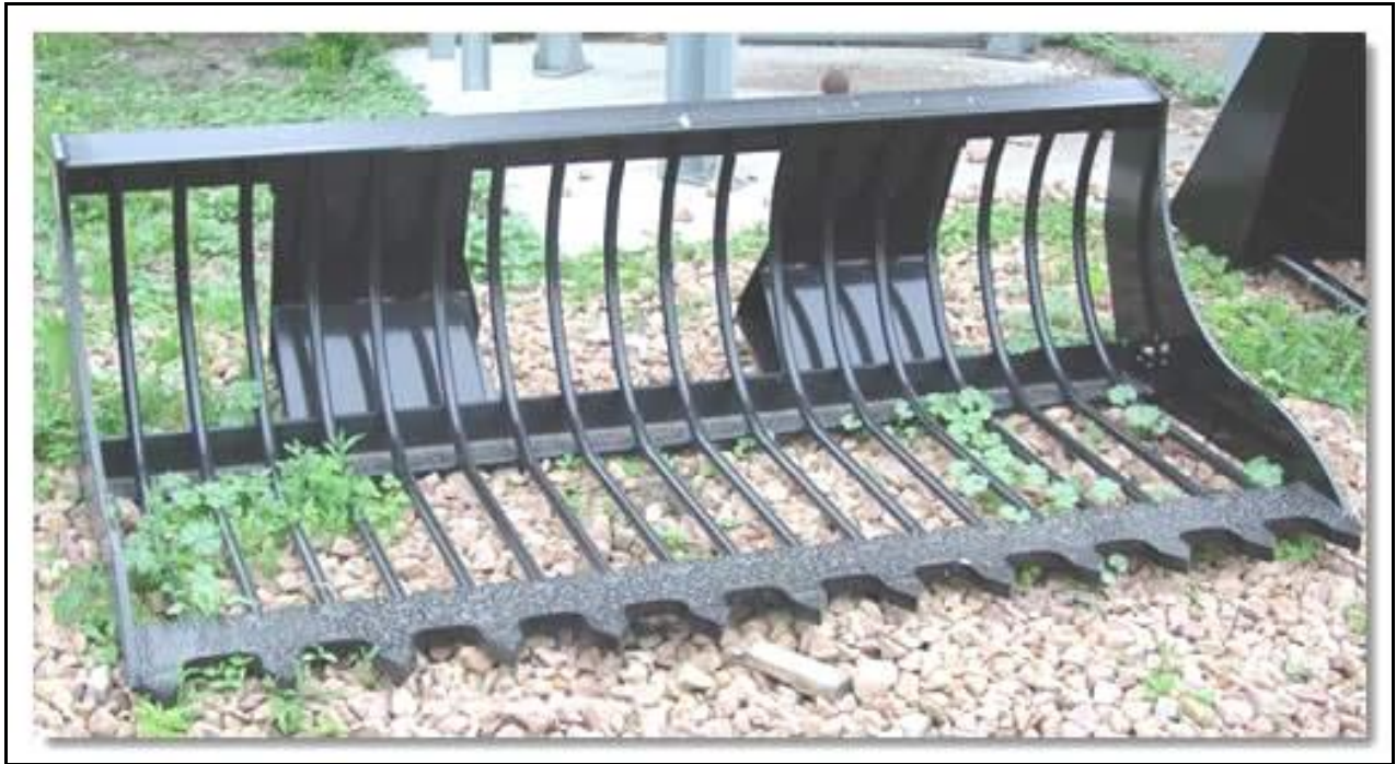
Figure 6. Example of a rock bucket to sort larger artifacts and sort rocks and debris.
