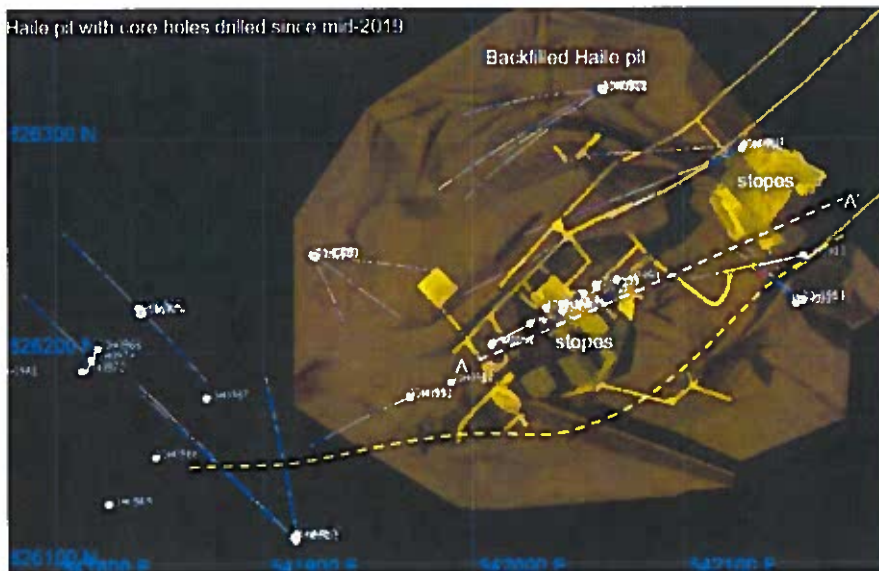
Figure 6: Site Map of Backfilled Haile Open Pit superimposed on documented underground workings Source: Haile – 2020
