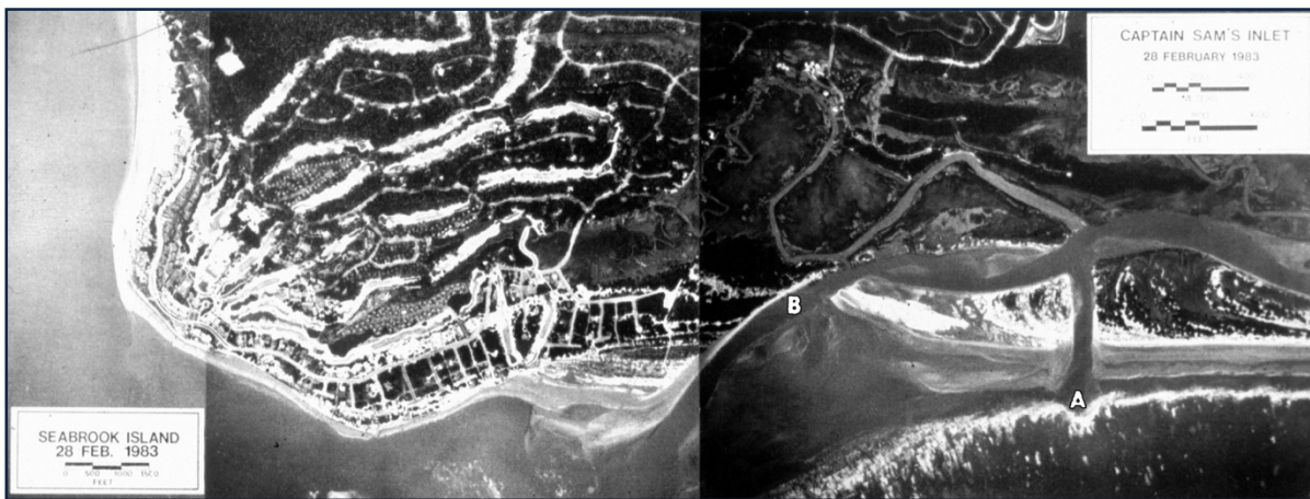
FIGURE T-3. Seabrook Island and Captain Sams Inlet in 1963 (upper) and 1983 (lower). The 1963 condition served as a model for the plan to relocate Captain Sams Inlet. Lower photo shows the new channel (A) open before the old channel (B) was closed on 4 March 1983.
