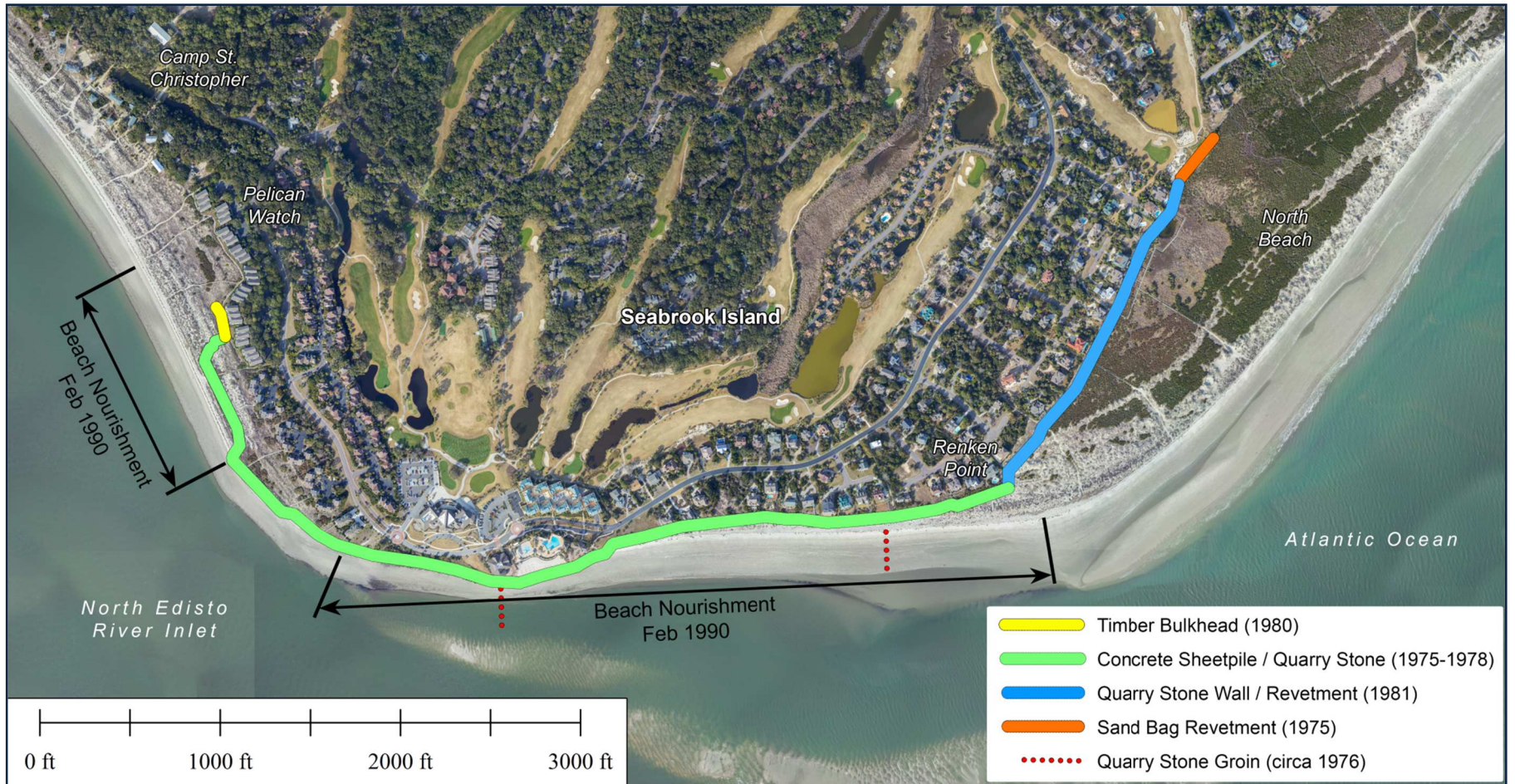
FIGURE 5.2a Location of shore-protection projects along Seabrook Island since the 1970s. Captain Sams Inlet relocation (1983, 1996, 2015) occurred between OCRM 2575 and the Kiawah/Seabrook Town easement line (outside image range, see Fig T-3).
