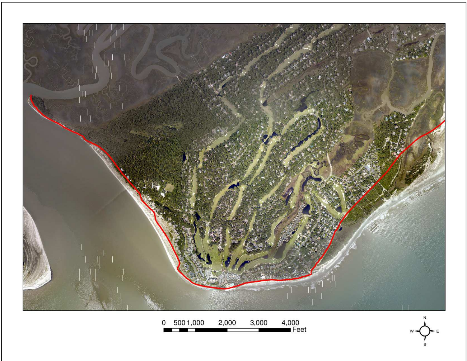
FIGURE 5.1k Official 2018 OCRM Setback Line for a portion of Seabrook Island superimposed on a 2019 rectified aerial orthophotograph. Image taken close to high tide.
