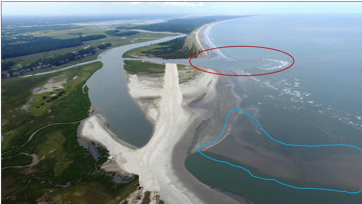
FIGURE T-12. Oblique aerial image of Captain Sams Inlet area from the Seabrook side in July 2015, following the third inlet relocation project. The ebb tidal spit along the east bank of the old inlet channel is clearly visible in the foreground (blue highlight), and the new channel’s associated ebb tidal delta is visible in the breakers adjacent to Kiawah Spit (red highlight).
